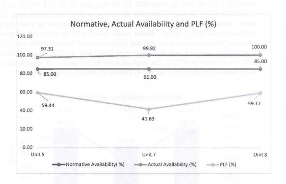
The entire monthly fixed cost was payable in line with MYT Regulations, 2019 as the cumulative plant availability of Unit 5, 7 and 8 were higher than the normative availability of 85%. It is observed that Unit 7 has lower PLF and lower generation resulting in higher fixed cost per unit than approved by the Commission. Also, the Variable Cost of the Units 5 and 8 was substantially higher than the approved cost
