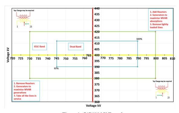
Figure 1: 765/400 kV Transformers
