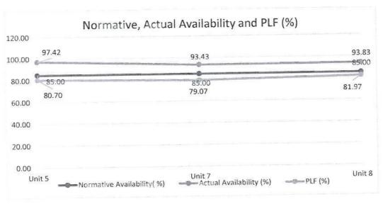
The entire monthly fixed cost was payable in line with MYT Regulations, 2019 as the cumulative plant availability was higher than the normative availability of 85%. It is observed that Unit 7 has lower PLF resulting in higher fixed cost per unit than approved by the Commission. Also, the Variable Cost of the Units 5, 7 and 8 was substantially
