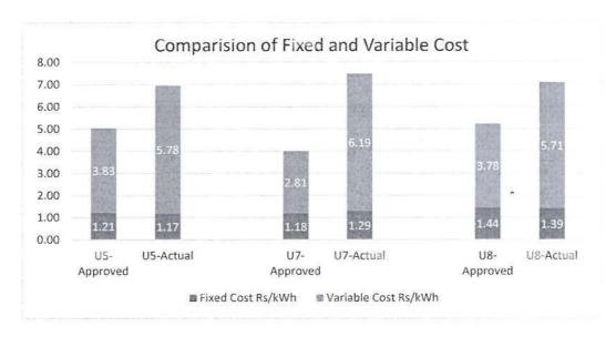
\*Unit 7 (APM+RLNG) actual rate is Rs.6.19/kWh as against approved rate of Rs. 2.81/kWh (APM). This is on account of the fact that due to shortage of APM gas, Unit 7 was also operated on RLNG in October 2021 which is costlier fuel whereas the approved rate of Rs. 2.81/kWh is based on APM gas alone which is a chepaer gas as compared to RLNG.
